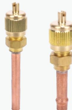
The charging valve is an one-way service valve with valve inside. The charging valve is used on the freezer; cold store and air - conditioning unit. Equipped with imported valve inside of reliable performance. Double sealing ensure leak-tight. Copper tube of various lengths and hardness are available. Valve bonnet is knurled for easy handling.
